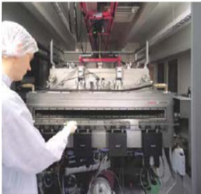
CIGS high throughput deposition up to 120 cm Substrate width
